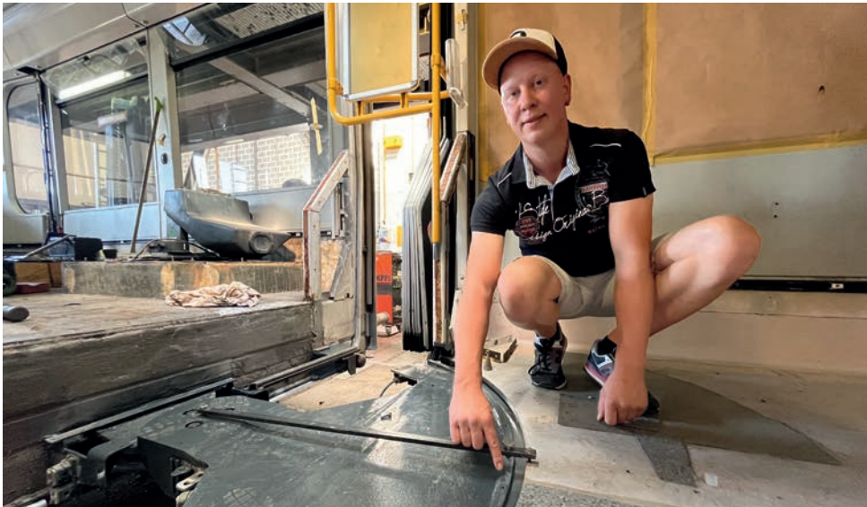
Tilo Ermlich shows off the welding gauge that allows precision welding.
